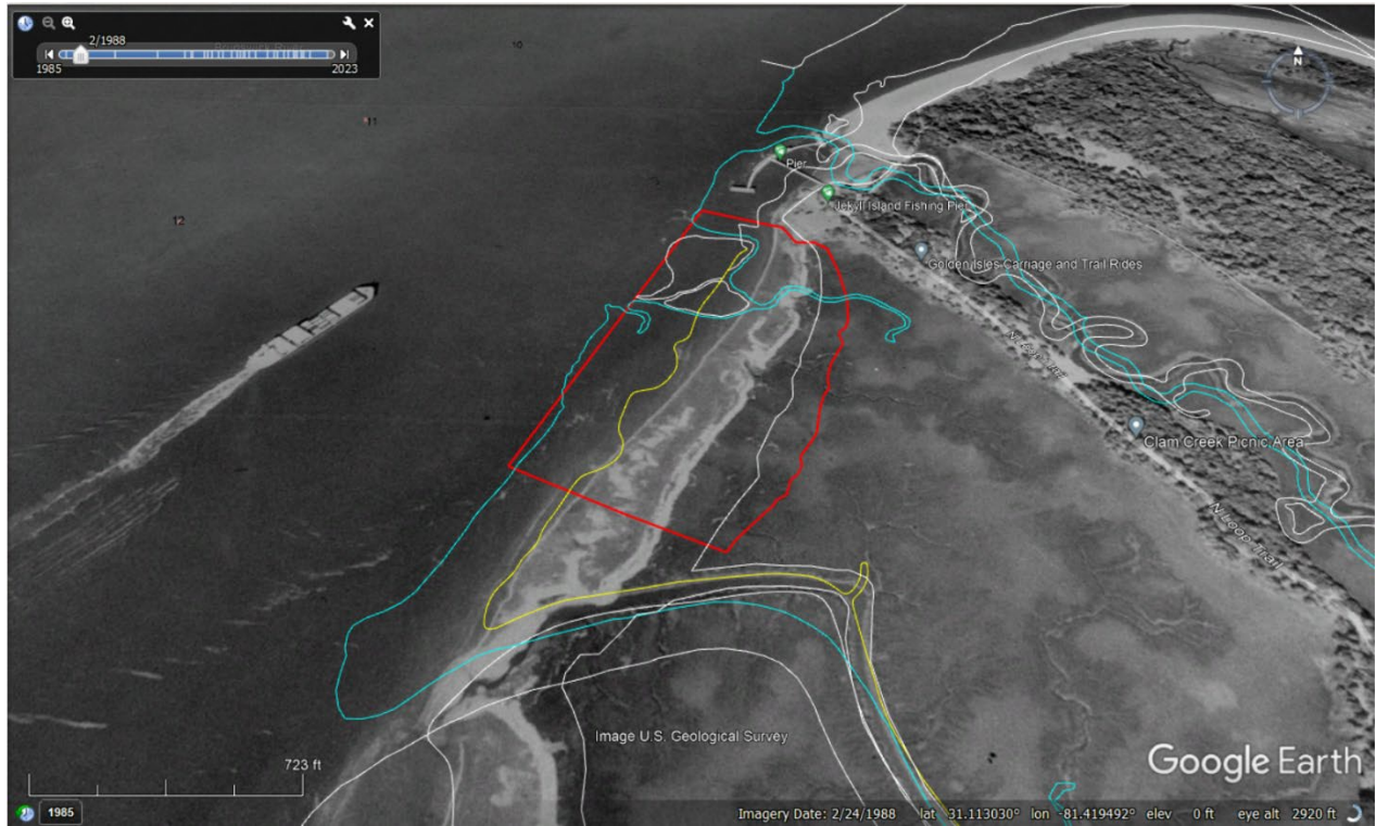
Figure 2. 1988 aerial imagery of the proposed placement location. The proposed placement polygon is in red. The blue line is historical shoreline from 1855, and the yellow is historical shoreline from 1933 (GADNR).
